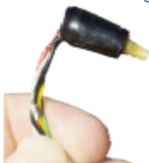
The original neonate probe designed in 1988 for the ILO88
