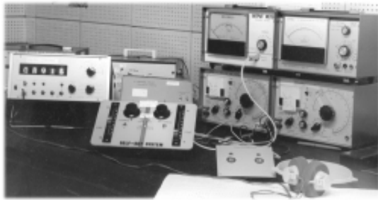
Kemp's psychoacoustic laboratory at the Royal National Throat Nose and Ear Hospital, London in 1975. Precisely calibrated oscillators delivered measured sound levels to ear via headphones. The listener manually adjusted level and frequency to map their auditory anomalies
