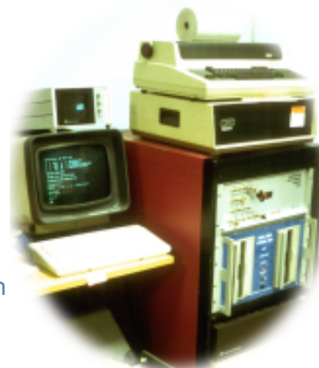
From 1981 the ILO laboratory OAE system was based on the 'SLAM' computer made by C.E.D. Ltd. The data analysis and presentation used on both the Peters AP200 (below) and ILO88 clinical OAE systems was developed on the 'SLAM'.
