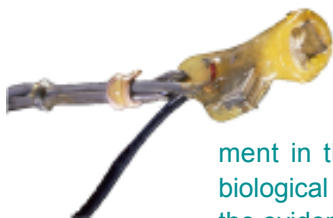
The first OAE probes were assembled from hearing aid parts and epoxy resin
